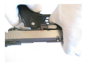
4. Press slide stop shaft on right side of fram and remove slide stop by pulling it out left side of fram. Then you can pull lide forwards from frame.
