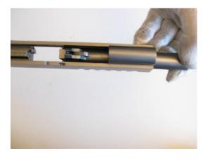
9. Assembly is done basically reversing order of disassembly. Install plug properly that front of plug lines with front side of slide.
