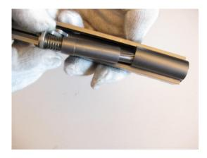
8. Tilt barrel link forwards and remove barrel through front of slide.
