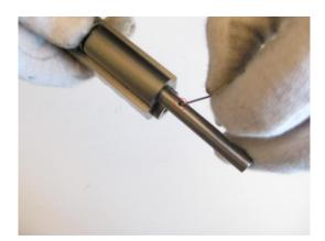
7. Let guide rod slowly come backwards until plug is touching the pin. Now you can remove rod, spring and plug together backwards.
