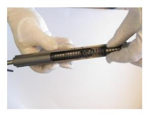
7. Using the bushing wrench, turn the bushing 1/8 turn center clockwise. Tilt barrel link forwards. Now you can take the barrel with bushing and plug through the front end of slide.
