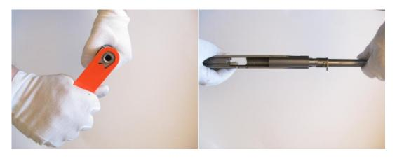
8. Assembly is done by basically reversing order of disassembly. Install plug properly that front of plug is centering the bushing.
