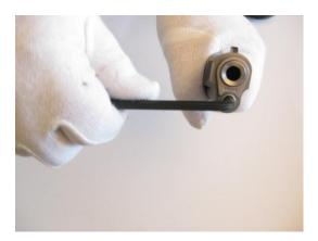
6. You can now carefully remove the front end of guide rod through front of slide and rear end with spring and plug through rear end of slide.
