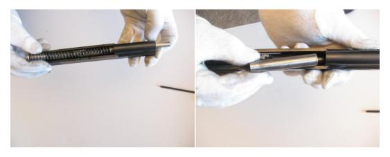
6. Tilt barrel link forwards and remove barrel through front of slide.
