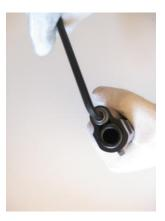
5. You can now carefully remove the front end of guide rod through front of slide and rear end with spring and plug through rear end of slide.
