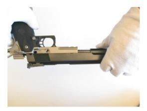
5. Put allen wrench into front of guide rod and open center-clockwise while fixing the end of the guide rod with other hand. **Please note that plug is under heavy tension from recoil spring.**
