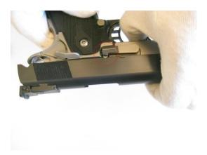
4. Press slide stop shaft on right side of frame and remove slide stop by pulling it out left side of frame. Then you can pull slide forwards from frame.
