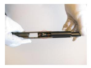
7. Assembly is done by basically reversing order of disassembly. Install plug properly that front of plug lines with front side of slide.
